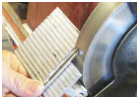
▲ Pic.2 Set the platform on the grinder so the bevel of the tool is a perfect match onto the wheel. I have cut away the platform on my grinder; this allows me to better position my hands
